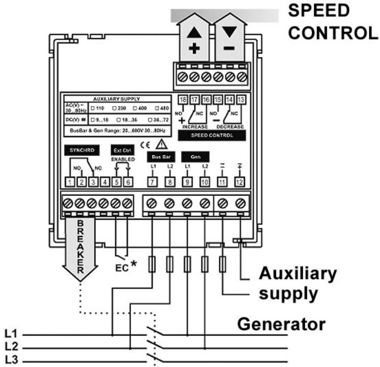
\* **EC (External Control):** The connection being opened disables the synchronisation relay (breaker)
