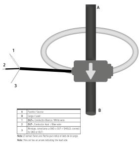
Note: The coil has an arrow indicating the load side.
