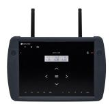
MYeBOX-1500, Portable power analyzer with recording of quality events and transients
