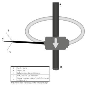
Note: The coil has an arrow indicating the load side.
