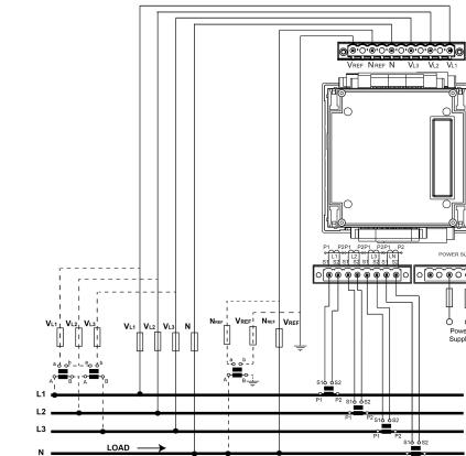
Measurement system: 4W-3 Ph (MC3 type transformer (.../0.25DA))
