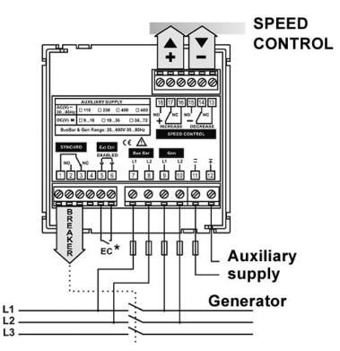
\* EC (External Control): The connection being opened disables the synchronisation relay (breaker)
