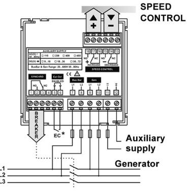
\* EC (External Control): The connection being opened disables the synchronisation relay (breaker)
