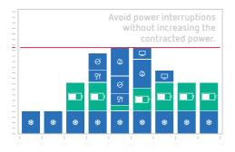
Compatible with the **CirBEON** sensor, which, combined with eNext, dynamically adapts the electric vehicle's consumption to the power available in the installation.
