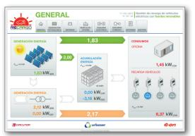
The general PowerStudio SCADA software screen was designed to represent the installation's block diagram and the status of the lines and units.
