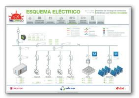
The "Electrical diagram" screen was intended to show a single-line diagram of the installation and to find out the main electrical parameters. It also offered a chance to see and act on the protection elements that could be operated in this way.
