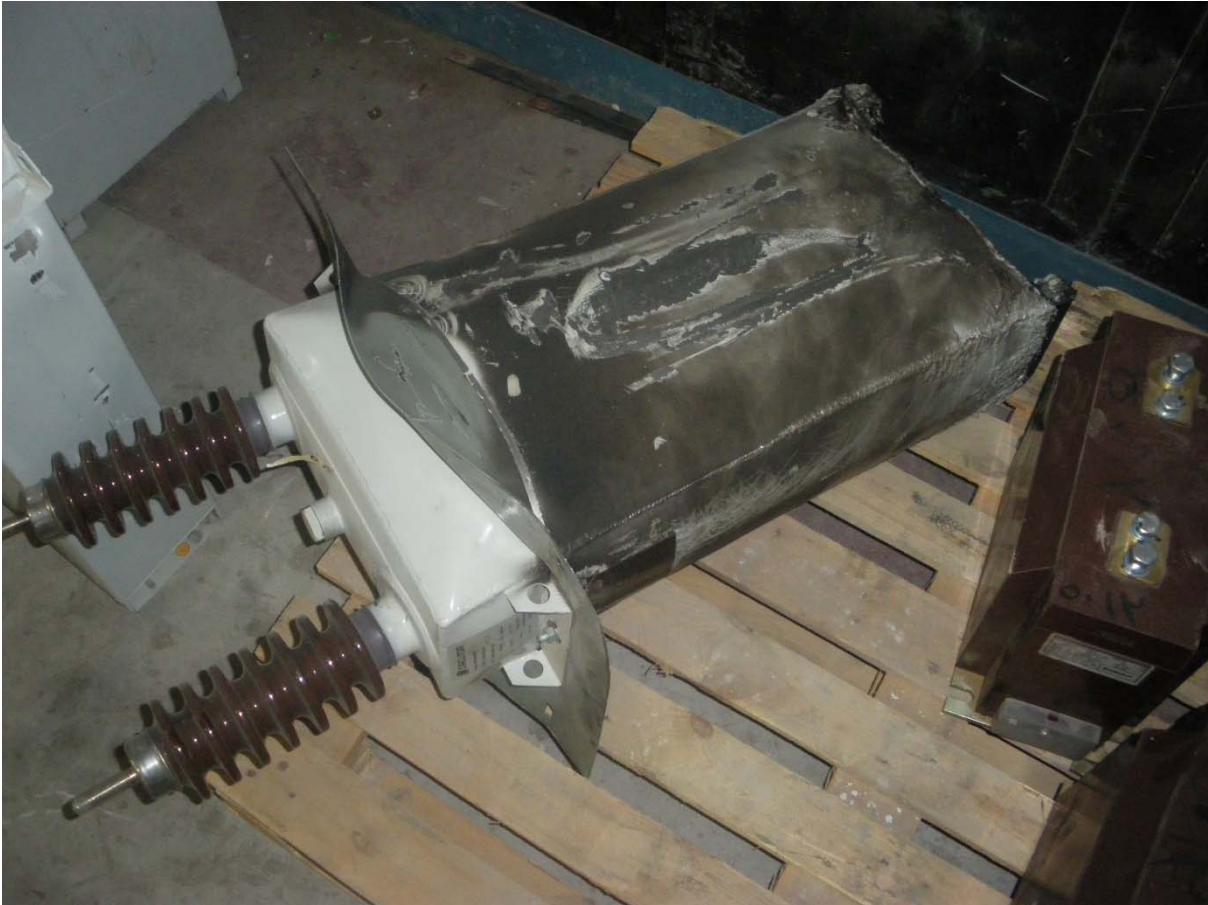
Image 1. Blow-up MV capacitor due a resonance effect
